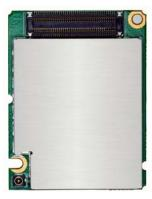
The **EDGE** Module new is а complete **Quad-Band** solution in a GSM/GPRS/EDGE compact plug-in module. interface. Featuring an industry-standard delivers GSM/GPRS/EDGE 850/900/1800/1900MHz performance for Data, voice, SMS, and Fax in a small form factor and with low power Consumption.
